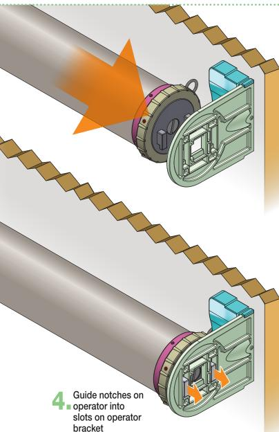
While pressing shade roller toward idler bracket, swing operator end of shade into position.
