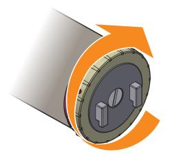
If shade does not stop but continues moving *DOWN*, adjust the spring force by turning adjuster ring *counter-clockwise* for Standard installations, and *clockwise* for Reverse Roll installations.
